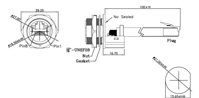
Panel Cut-Out Panel Thick:1.5~4.5mm
