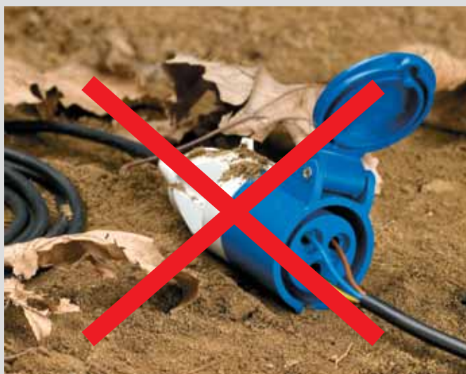
Connector tube protective shutter for greater safety against direct contacts. (The SAFE-IN safety device).
