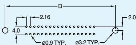
RECOMMENDED PCB LAYOUT (TOP VIEW)
